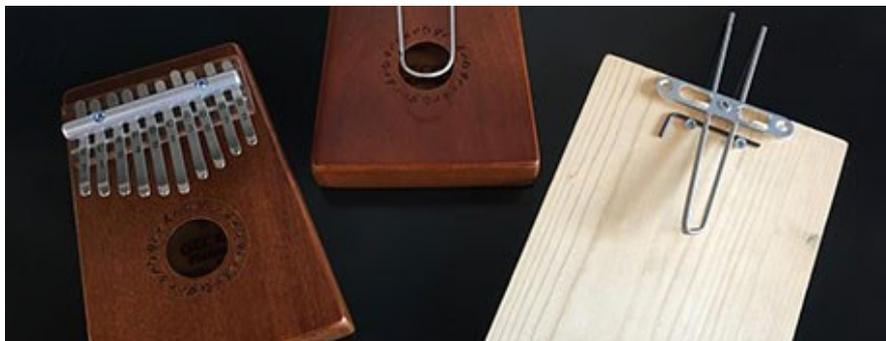
Inspired by a musical instrument, the simple sensor can be constructed from common materials and used to detect adulterated or counterfeit drugs.
