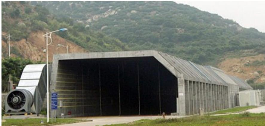
Road tunnel fires are mainly caused by vehicles and their load. The researchers thus set fire to gasoline and diesel to simulate oil surface burning caused by fuel leakage following vehicle collision.
