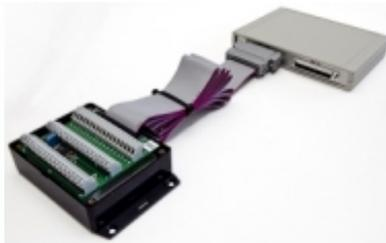
*[A cold-junction measuring box connected to data acquisition hardware](#)*
